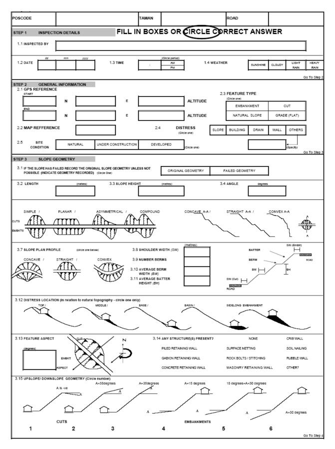
Figure 2a: Shows the format and content of slope proforma page 1 of 3
