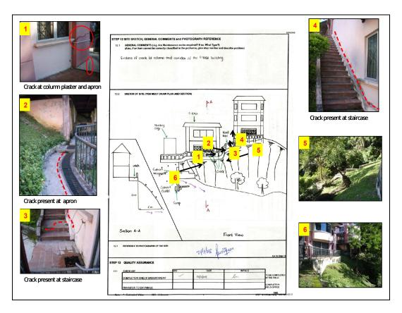
Figure 3: shows an example of field geomorphological survey done for a soil slope, with a bungalow on top of slope showing signs of distress, with cracks on apron slopes and columns.
