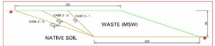
Figure 38 : Case 2 - Landfill of 30m high (H) and 120m width (W), W/H = 4
