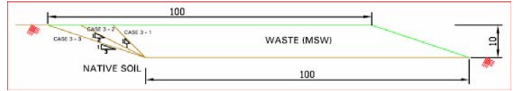
Figure 39 : Case 3 - Landfill of 10m high (H) and 100m width (W), W/H = 10
