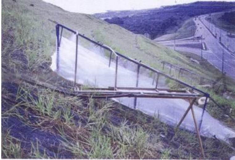
Figure 3. Rainfall simulation in progress
